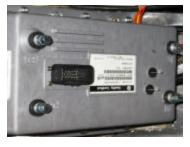
3.) Connect the wire labeled "A1" to the control terminal labeled "A1" using the supplied M6 -1.0 X 25MM bolt (HW B M6 X 25MM), M6 lock washer (HW L M6), and flat washer (HW F M6) with 10mm socket. See **Figure 7**.
